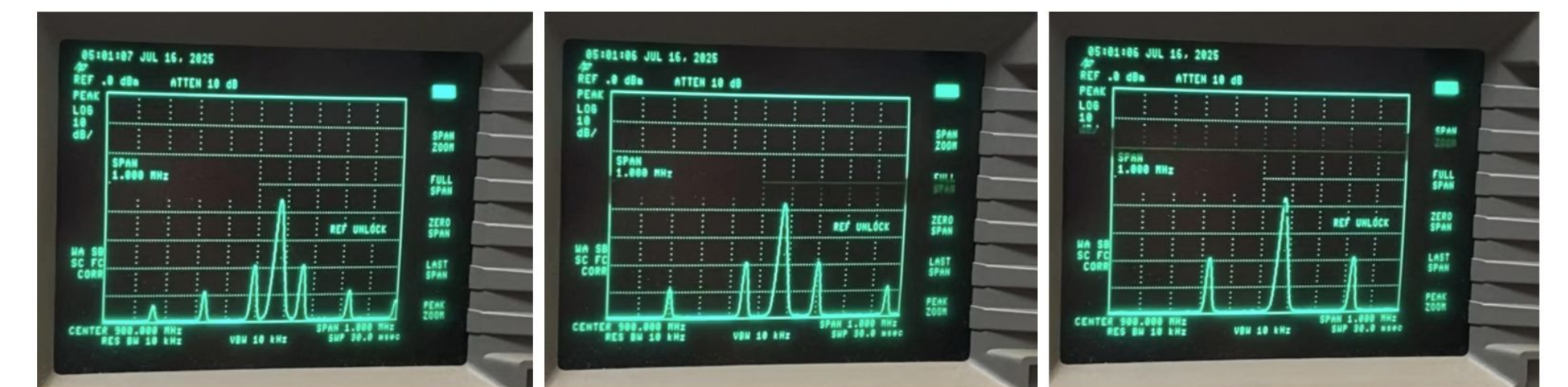
Figure 5: Photos from Spectrum Analyzer Demonstration of Frequency Shift Keying (FSK)
